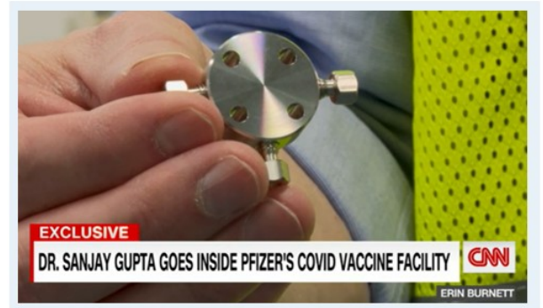
"T-Mixer" used to create LNP; Arbutus/Genevant '320 patent
